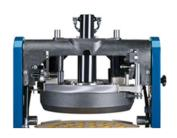
Low-pressure dividing system respects the dough and requires no physical effort from the operator. The DR Robot is equipped with reliable and proven electronics and silent, specially engineered long life hydraulics.
