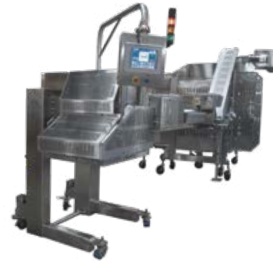
Sani-Chain Collator with Lower, Easy Access Removable Flights
