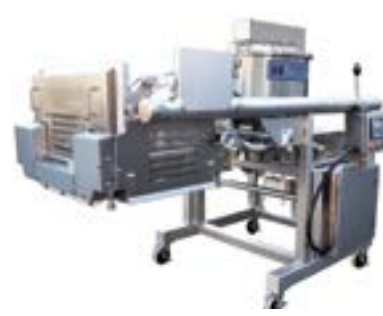
6 Piston Servo Filler with Bridge & Hopper Agitator
